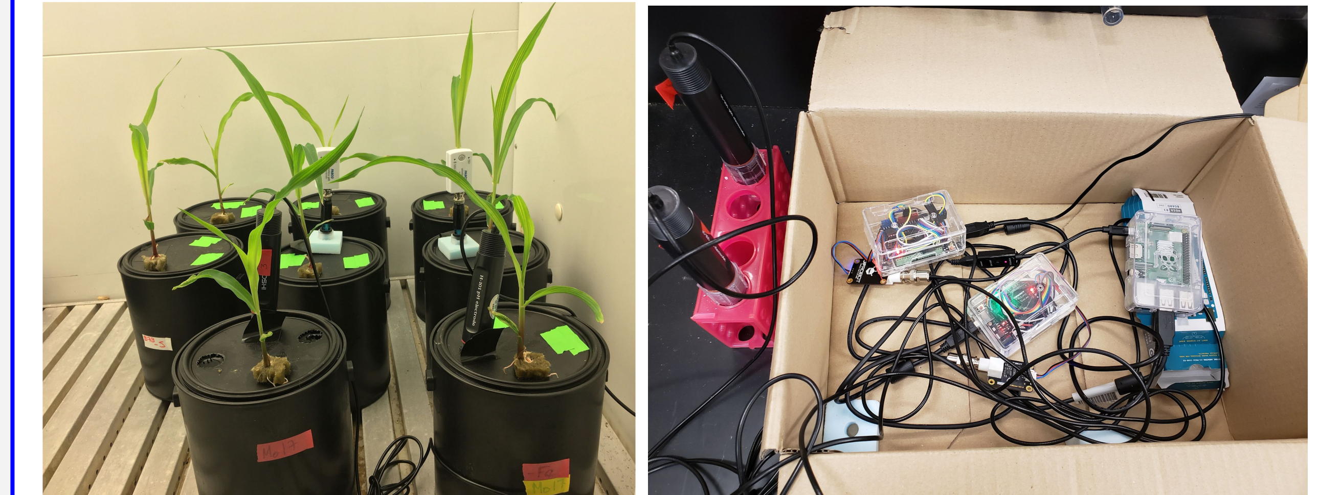
Figure 2A and 2B Maize Setup: 4 total maize plants were grown hydroponically in a growth chamber. A cutout on the lid of the canister containing the hydroponic solution allowed the pH sensor to rest in the solution to take continuous data. 2B shows the electronics setup for the DFRobot sensors. See video LusardiAndWalter for more details.
