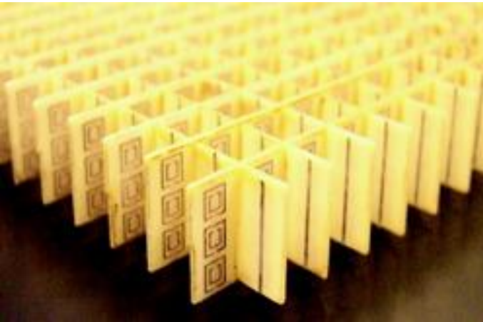
A photonic metamaterial that displays a negative refractive index.
