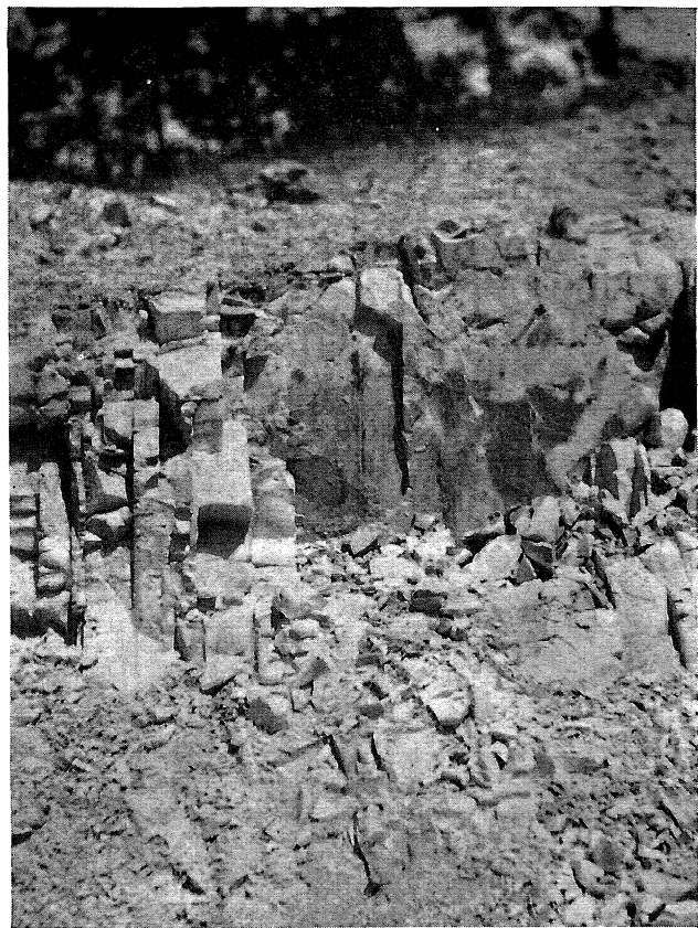
A. Vertical jointing in flint fire clay, Fisher pit, north of St. James, Phelps County.
